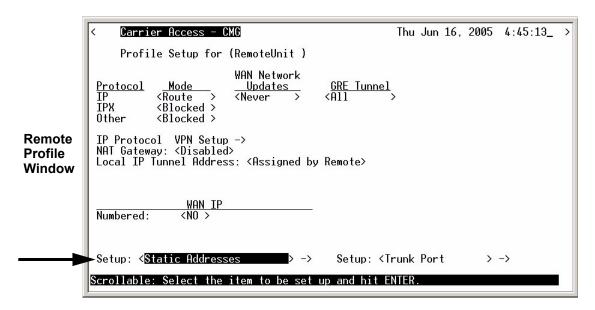
4. Select **Setup: Static Addresses >**, scroll through the list of options with the **[SPACEBAR]** if **Static Addresses** is not displayed. Press **[ENTER]**.
